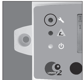
System fault indicator
