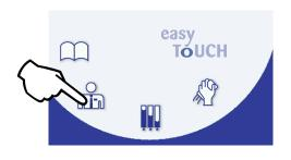
After selecting Manager's Menu icon from the Main Menu, the password screen appears. The manager screens are password protected. (Default Password is "A".) Enter the Manager's pass code using the QWERTY keypad, then press the green check to accept.
